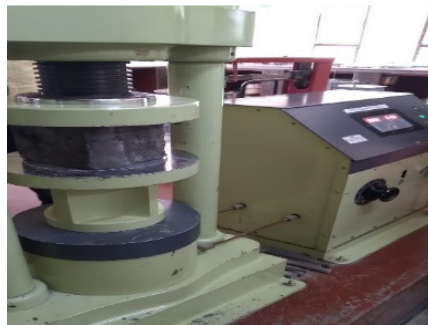
Fig 1:Testing of cube
