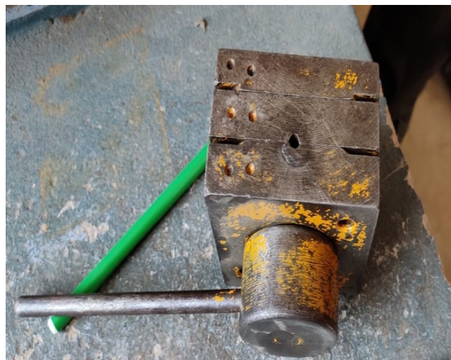
Fig 3: Mild steel Die for manufacturing Cap
