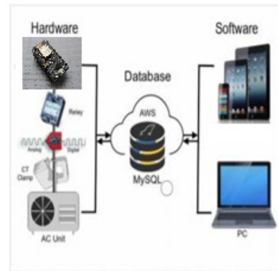
THE ARCHITECTURE DIAGRAM OF THE IOT MONITORING AND CONTROL SYSTEM
