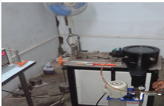
Figure 1. “Test Setup “Pin on Disc Tribometer”
