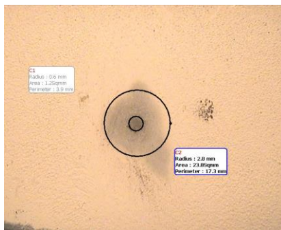
Fig. 6 Stereo micrograph of abraded surface
