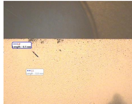
Fig. 7 Stereomicrograph of Scratch test sample
