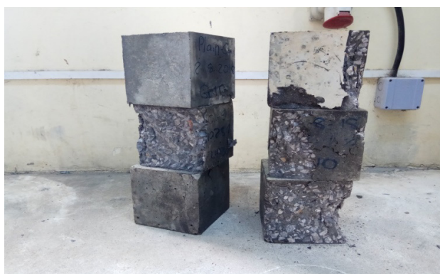
Figure 2: Compression of Concrete Cube Specimen after Compressing
