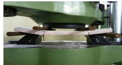
Fig -4: Flexural Test
