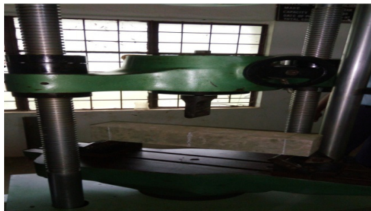
Fig 3 Flexural Test On Nominal Mortar
