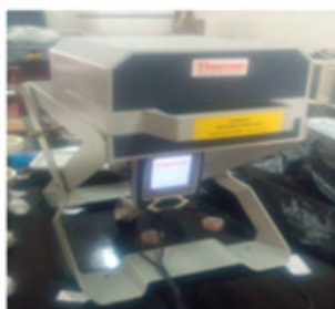
FIGURE 2: EDXRF used for elemental analysis of powdered plant sample
