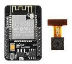
**Role**: The ESP32-CAM module serves as the "brain" for controlling the surveillance camera functionality of the robot. The camera is useful for capturing video or images for surveillance purposes.
