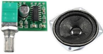
Fig 5. PAM8403 Audio Amplifier & Speaker
