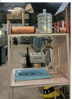
Fig: Water saving toilet flushing system
