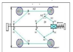
Static Analysis: In order to decide the actuator size, it is necessary to perform the static analysis. Assume that in Fig., Fcx and Fcz denote the reaction force and the traction force exerted on the four-bar by the driving wheel, respectively. Now applying the virtual work principle to the free-body diagram gives:
