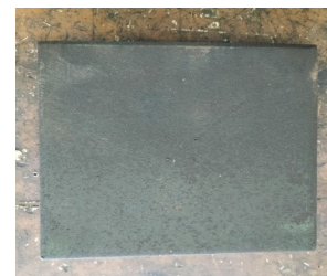
Fig.8 Model square footing
