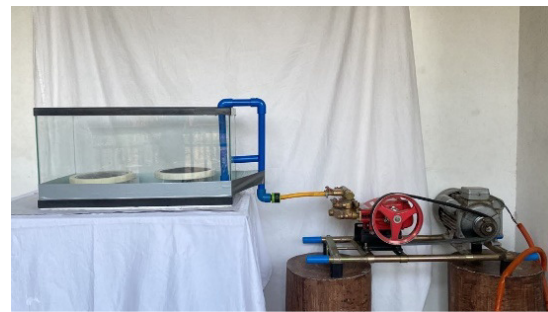
Fig 6 Front View of the Actual Prototype Aeration Set-Up
