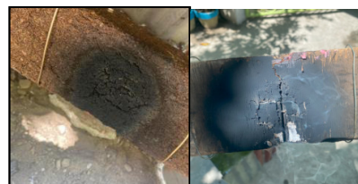
Figure 18. Fiberboard Composite Mixture and Plyboard Sample after Ignition
