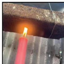
Figure 16. Fiberboard Composite Mixture Samples During Direct Heat
