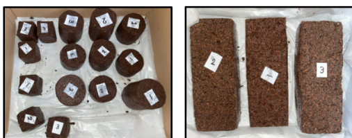
Figure 7. Saturated Fiberboard Specimens
