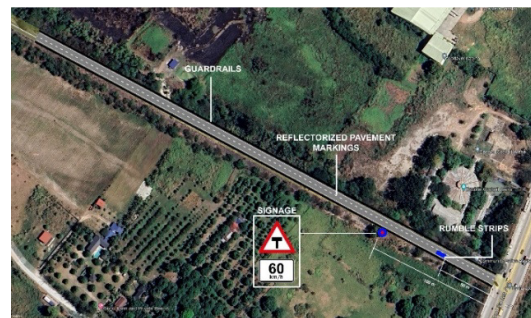
Fig. 9 2D View of the Proposed Countermeasure II on Segment 1
