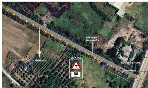
Fig. 23 2-Dimensional Layout Plan of Proposed Countermeasure for 2nd Black Spot Priority (Segment 1: K0+000 - K0+500)
