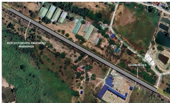
Fig. 22 2-Dimensional Layout Plan of Proposed Countermeasure for 1st Black Spot Priority (Segment 5: K2+000 - K2+500)
