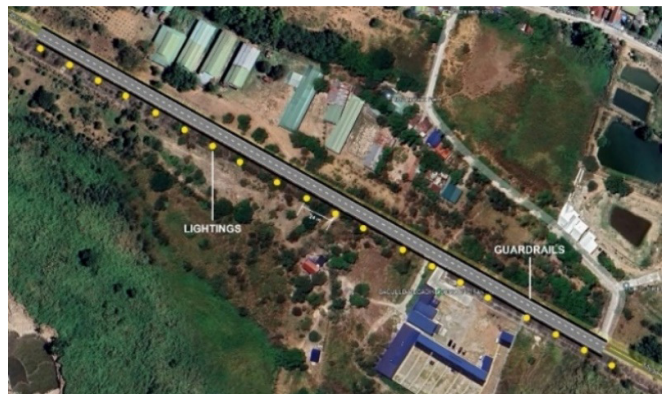
Fig. 5 2D View of the Proposed Countermeasure I on Segment 5
