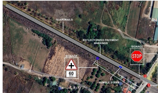
Fig. 12 2D View of the Proposed Countermeasure II on Segment 12
