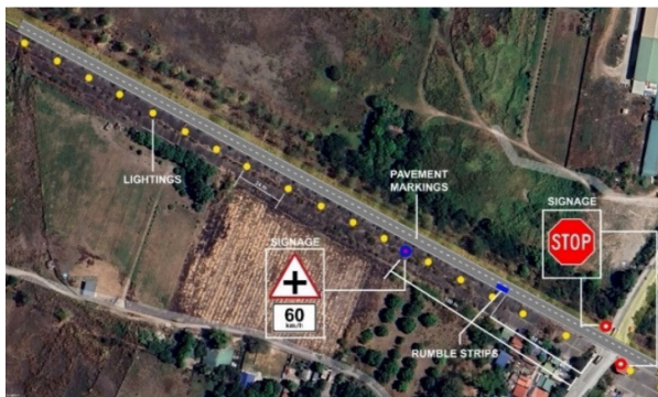
Fig. 11 2D View of the Proposed Countermeasure I on Segment 12
