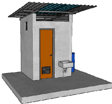
Fig. 13 3-D Model of One-Section Sanitation Facility
