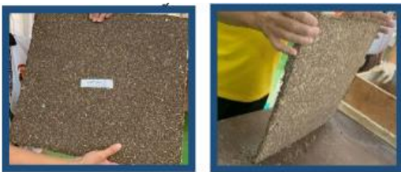
Figure 6. Solidified Particleboard After Hot Pressing
