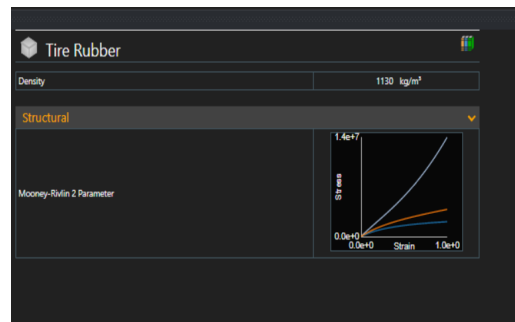
Fig. 4. Material Property of Tire Rubber used in ANSYS Workbench The researchers used a density of 1130 kg/m 3 for the tire rubber using the Mooney-Rivlin 2 parameter as the basis for its hyper elasticity. This
