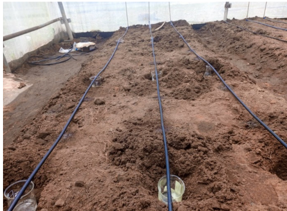
Figure 4: Flow measurement of emitter discharge at pressure head of 1.5 m
