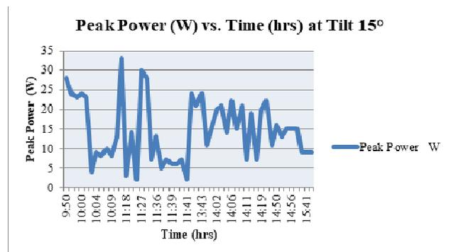
Fig. 9 Peak Power (W) vs. Time (hrs.) at Tilt 15°
