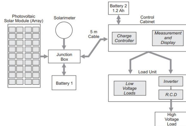
Fig. 2 Configuration of Photovoltaic System
