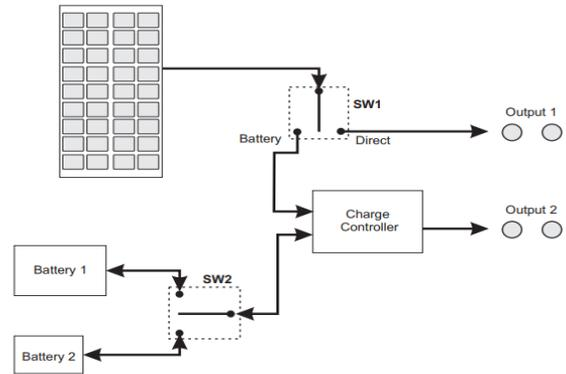
Fig. 3 SW1 and SW2 Circuits
