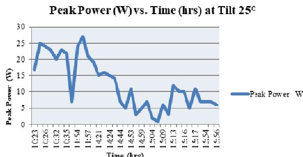
Fig. 11 Peak Power (W) vs. Time (hrs.) at Tilt 25°
