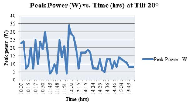
Fig. 10 Peak Power (W) vs. Time (hrs.) at Tilt 20°
