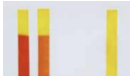
Positive Negative Fig. 1 The results of borax detection were positive and negative, respectively.
