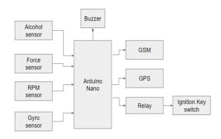
We use Arduino nano main controllers, sensors are Alcohol sensor, Force, RPM for speed, Gyro for axis. GSM for SMS, GPS for coordinates and Relay for ignition switch and Buzzer.
