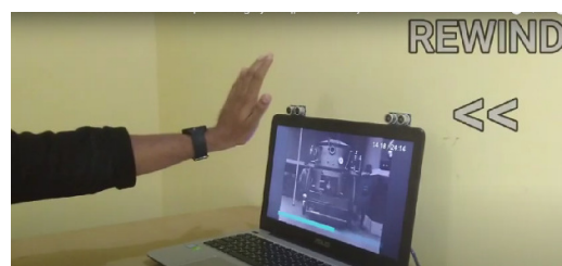
Fig10 : Represents rewind feature using hand gesture
