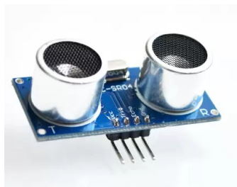
Fig2: HC-SR04 Ultrasonic Sensor
