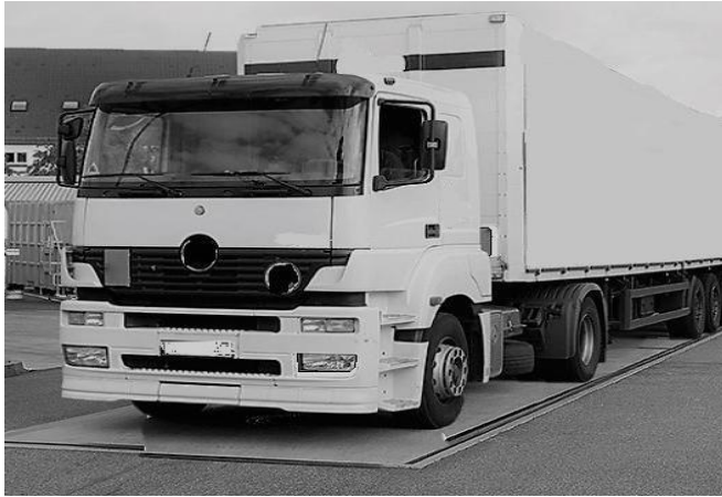
Fig.5. Truck resting upon floored load cell
