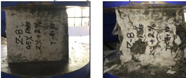
Figure 11 testing of concrete samples
