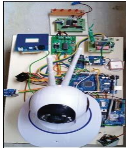
Figure 7. Activation of GSM for Sending SMS when metal is detected
