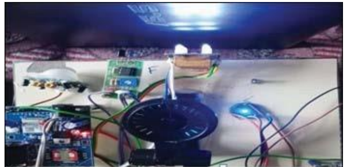
Figure 8. When colour sensor detects the color in front of it, then RGB turns to that identified color.
