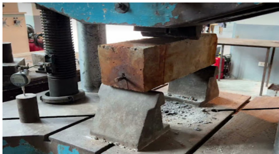
FIG. VIII STANDARD TEST METHOD FOR FLEXURAL STRENGTH OF CONCRETE
