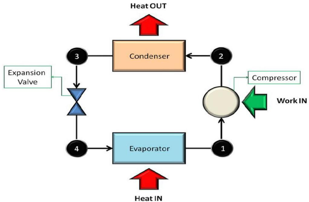
dehumidify warm air. After heat and mass are transferred, the lower temperature and lowerhumidity air is sent to the air-conditioned space to balance heat and humidity load of airconditionedspace.Itshouldbeobservedthatthesystemoperatesona closedcycle. Thesystemrequires input in the form of mechanical work. It extracts heat from a cold space and rejectsheattoahightemperatureheatsink.
