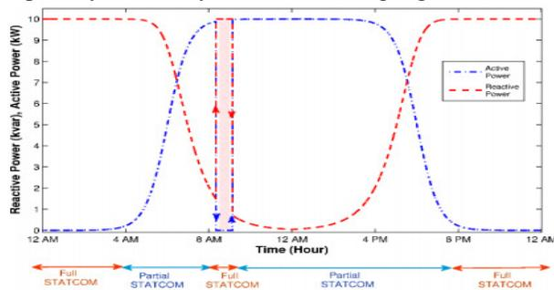
Fig. 1. Concept of smart PV inverter control as STATCOM (PV-STATCOM)
