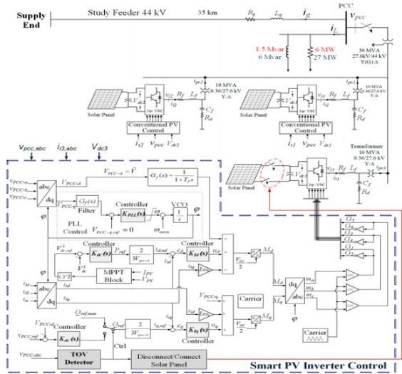
Fig. 3. Modeling of the study system and control components
