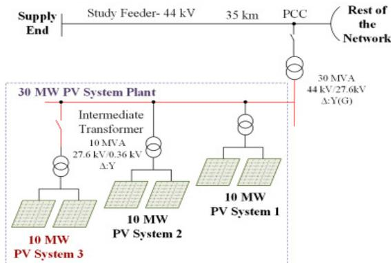
Fig. 2. Single line diagram of the study system
