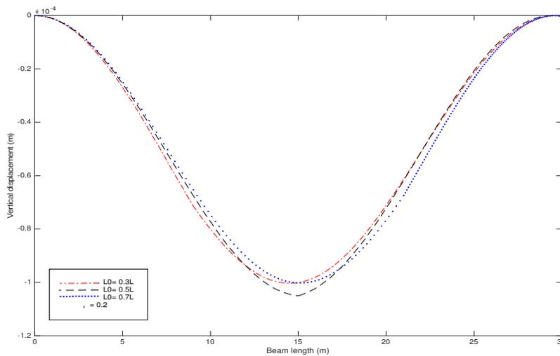
**Figure 5.** Vertical displacement with respect beam length with various crack position
