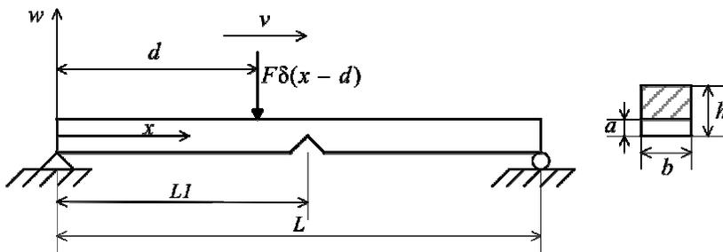
Figure 1. A simply supported cracked beam under concentrated force
