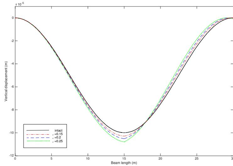
**Figure 4.** Vertical displacement with respect beam length with various crack depth ratio
