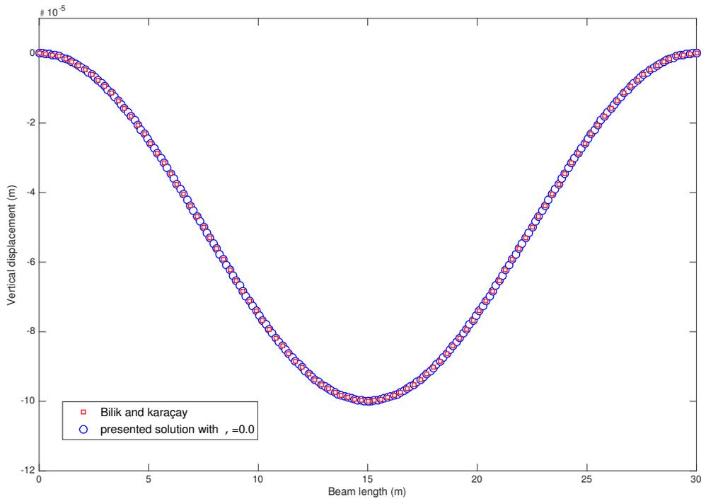
**Figure 3.** Comparison of the results of the presented study with Bilik and Karaçay for intact and cracked simply-supported beam subjected to concentrated force when  $\alpha = 0.0$
