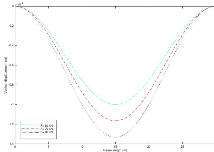
**Figure 6.** Vertical displacement with respect beam length with various forces( $\alpha = 0.2$ )
