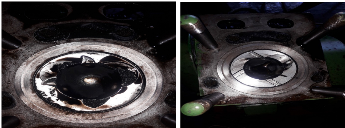
Figure 2.3 Modified Beak and Tangential Grooved Pistons After Combustion
