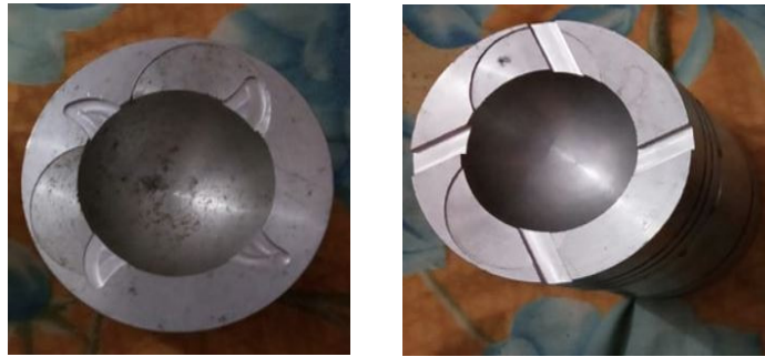
Figure 2.1 Image of Beak and Tangential Grooved Pistons Before Placing into Cylinder
