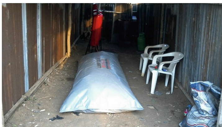
Figure 3 A gas storage bag filled with non-condensable pyrolysis gas
