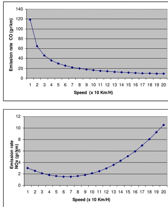
Fig 1. Relationship between Exhaust Emission Rate and Speed
