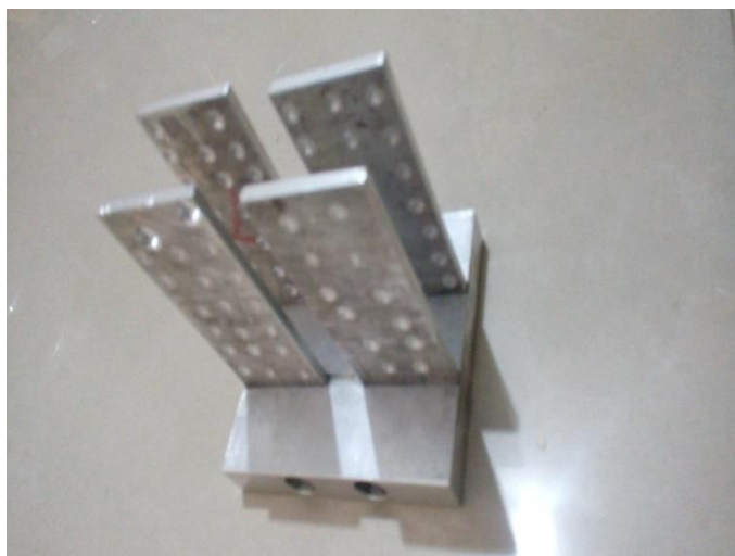
Fig:1. Dimpled fins 2x2 array fixed on heater base
