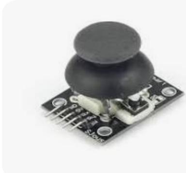
Figure 10-Joystick Module
