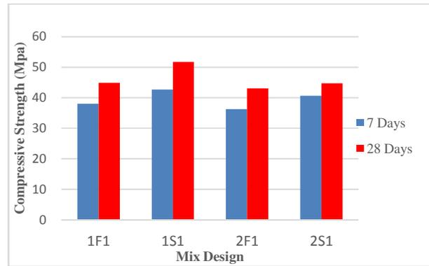
Fig. 3 Compressive Strength for 7 and 28 days cluster one mixes
