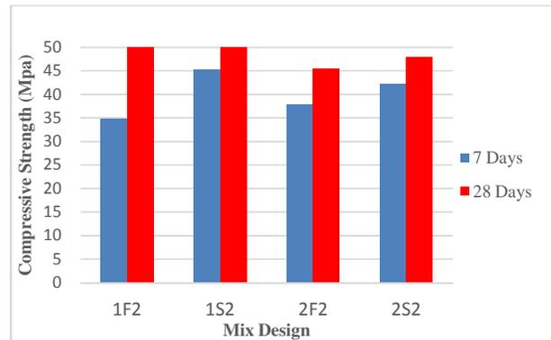
Fig. 3 Compressive Strength for 7 and 28 days cluster combination of mixes
