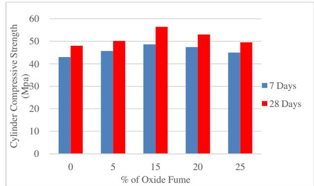
Fig. 2 Cylinder Compressive Strength for 7 & 28 days
