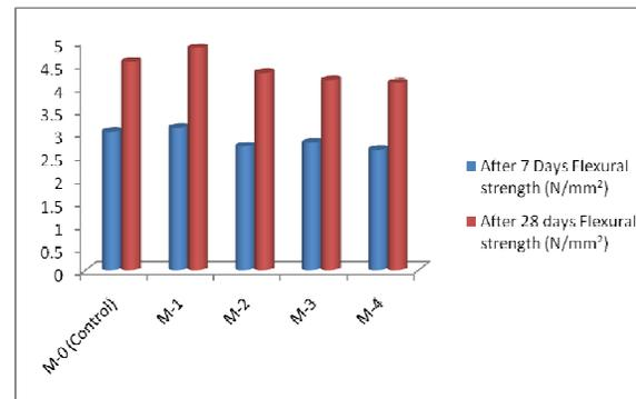
Fig. 4. Comparison between 7 and 28 days Flexural Strength
