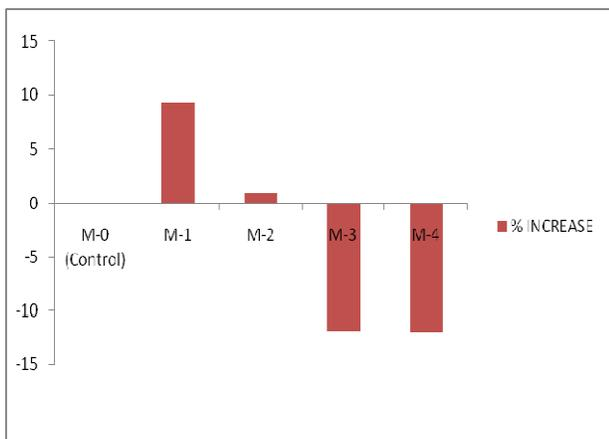
Fig. 4 % variation in Comp. strength relative to controlled mix after 28 days
