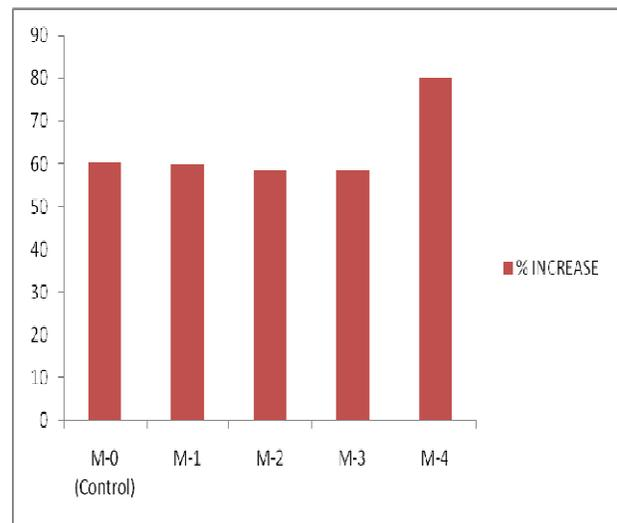
Fig. 2 Comp. strength relative to controlled mix after 7 days
