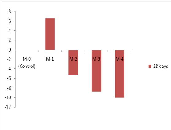
Fig. 7. % variation in flexural strength relative to controlled mix after 28 days
