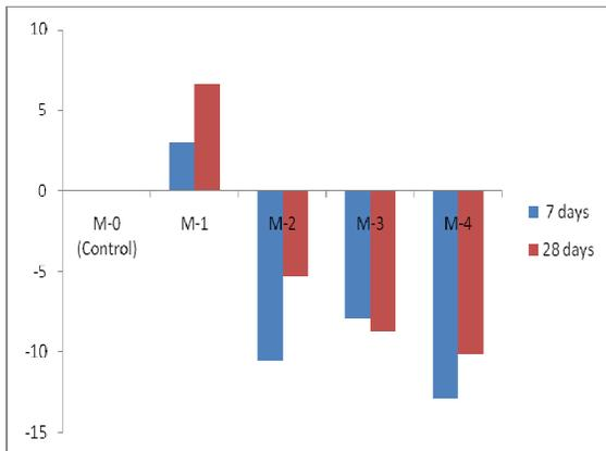
Fig. 8. Comparison between 7 and 28 days % variation in Flexural Strength
