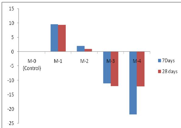
Fig. 5 Comparison between 7 and 28 days % variation in Compressive Strength
