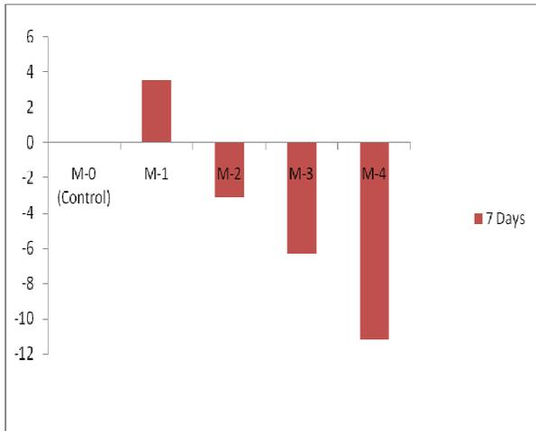
Fig. 1. % variation in Split Tensile strength relative to controlled mix after 7 days
