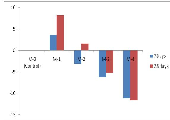
Fig. 3. Comparison between 7 and 28 days % variation in Split Tensile Strength
