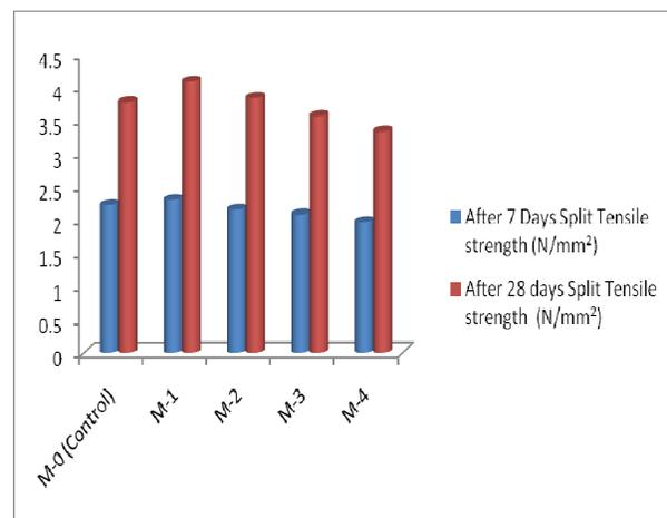
Fig. 6 Comparison between 7 and 28 days Split Tensile Strength
