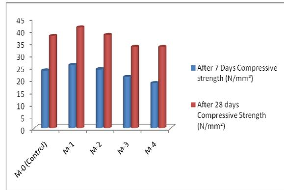
Fig. 1 Comparison between 7 and 28 days Compressive strength
