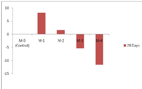
Fig. 2. % variation in Split Tensile strength relative to controlled mix after 28 days
