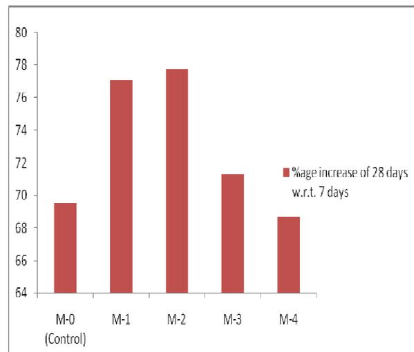
Fig. 7 Percentage increase in Split Tensile strengths of 7days to 28 days
