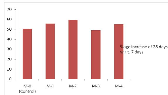
Fig. 5. Percentage increase in flexural strengths of 7days to 28 days
