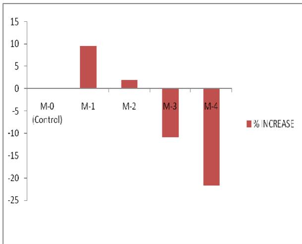
Fig. 3 % variation in Comp. strength relative to controlled mix after 7 days
