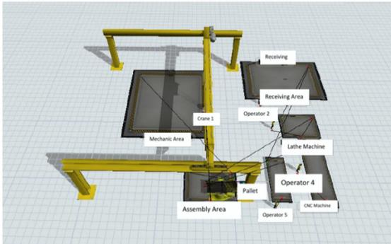
Fig. 6 Flexsim Simulation Layout CORELAP Algorithm
