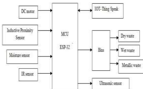
IR sensor senses whether the waste bin is filled or not. If the bin is filled, then the IR sensor gives information to the microcontroller. Then according to the coded program in the microcontroller, after a delay of 5 seconds servo motor rotates the waste bin in 120° and hence allows the wastes to fall onto the sub-conveyor. It starts to roll. Now the wastes are falling onto the main conveyor. Based on the
