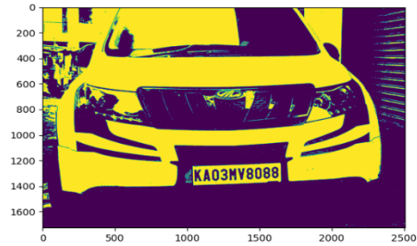
Figure 4: This shows the image after undergoing all the Morphological operations like dilation, opening and Erosion.
