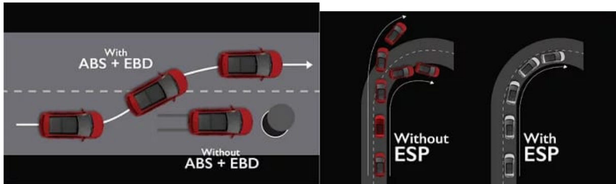
Figure 7. ABS with EBD & Corner Stability Control
