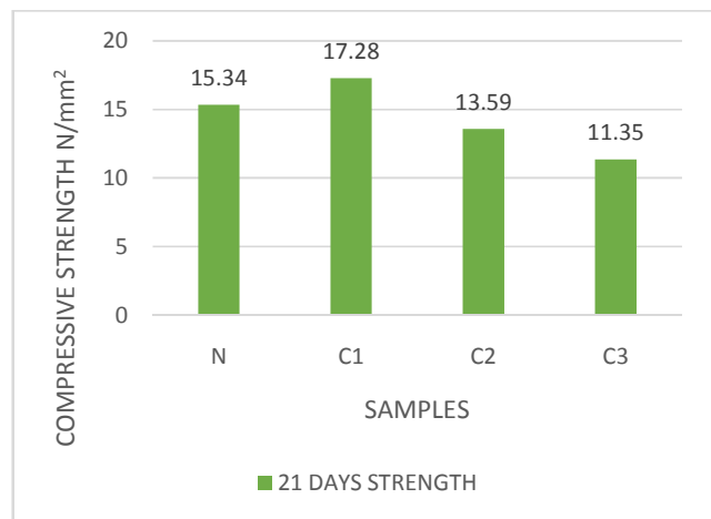
Graph 6:- Graph showing compressive strength of brick after 21 days of curing in partial replacement of cement with ggbs
