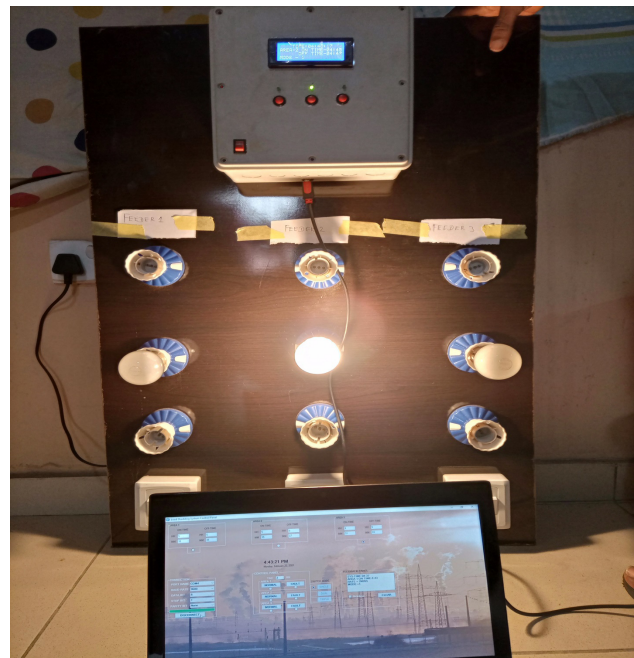
Fig.3: The load shedding system operating in single mode with feeder one ON.
