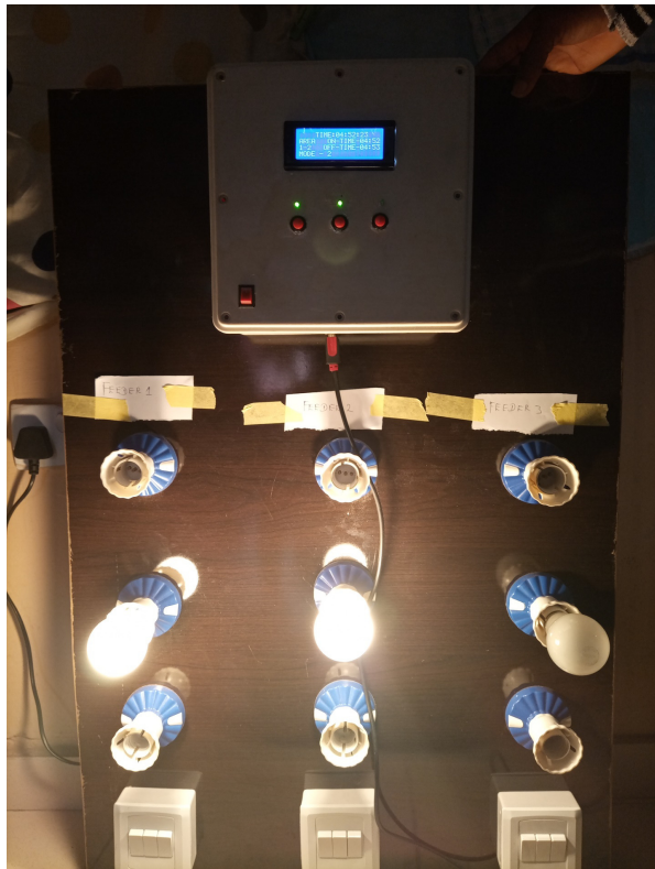
Fig.4: The load shedding system operating in dual mode with feeders one and two ON
