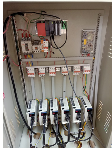
Fig 4 VNREDSat-1 hexapod control system
