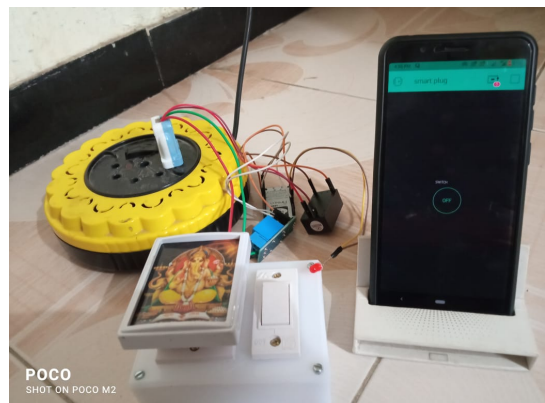
Fig 9: Before Output (Blynk App Button on Mobile Phone Turned Off)
