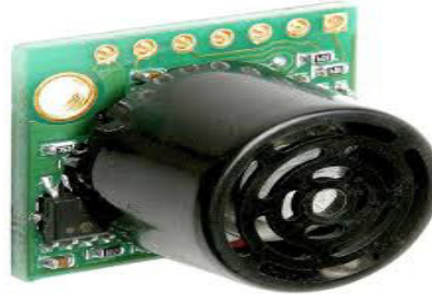
Fig 2 LV – Max Sonar MB1010
