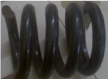
fig.1.1 broken helical coil spring
