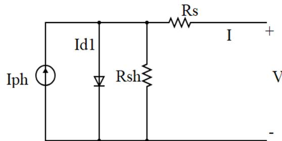
Fig1. Circuit of single diode photovoltaic model
